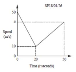
The train slows down uniformly from a speed of 50 m/s to a speed of 10 m/s in a time of 20 seconds.
