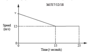
The car slows down uniformly from a speed of  $\nu$ m/s to a speed of 12 m/s in 15 seconds. It then travels at constant speed for a further 10 seconds.
